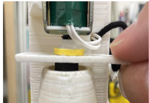
Figure 6 Spacing adjustment between solenoid and button
